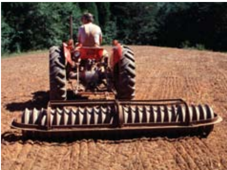
Fig. 4.11 A cultipacker is the best implement to firm a seedbed prior to sowing small seed (such as ladino white clover) and to establish firm seed-to-soil contact after sowing. Some folks use a section of chain-link fence to smooth a plot and reduce clods prior to planting. This can lead to better seedbed, but it is not a replacement for a cultipacker, which is needed for firm seed-to-soil contact.
