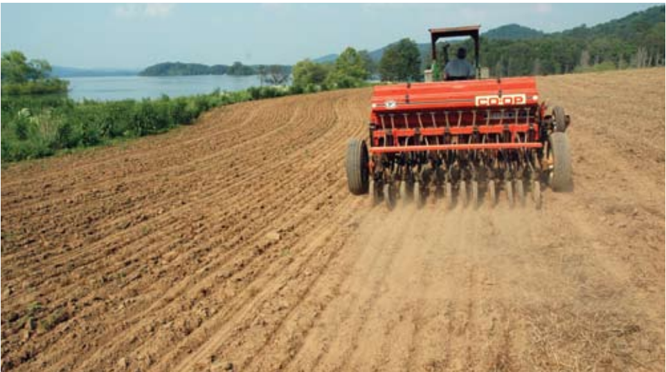
Fig. 4.8 Drilling seed is a most reliable planting technique. All seed are easily planted at the desired depth and germination rates are higher, thus less seed is required per acre.
