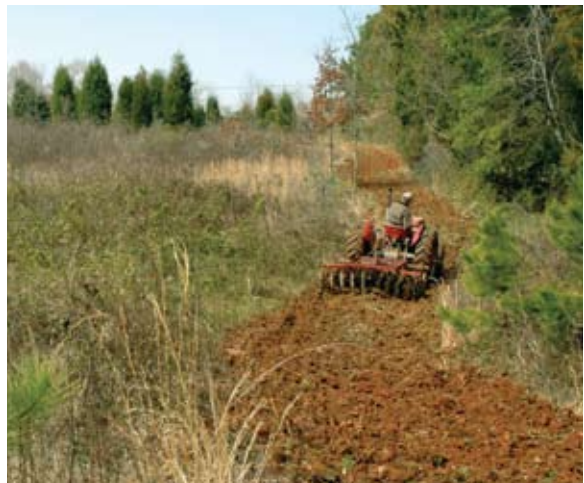
Fig. 9.1 Firebreaks are easily established around fields with a tractor and disk.
